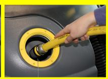
A Open the cover of the fresh water reservoir. Fill in fresh water (maximum 60 °C). Leave sufficient space for the detergent.
